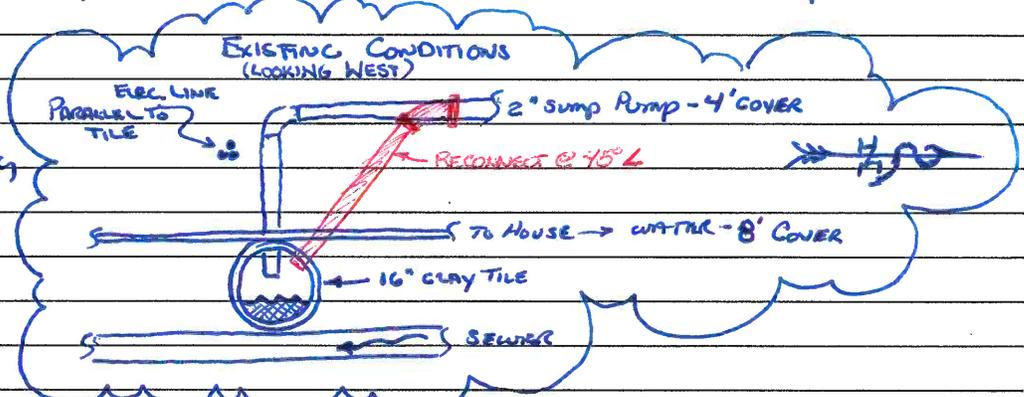
11:00 A.M., WATER LINE IS CUT AND OUT OF WAY. 12:00 Noon; TILE EXPOSED, 48" OF 18" HOPE DUAL WALL SET IN PLACE WITH FABRIC AND MESH FOR COLLARS. 2:00 DOWN WITH 1" CLEAN ROCK.
